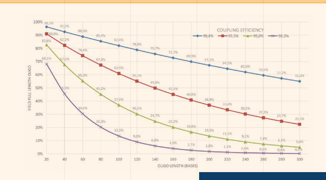
Figure 2 | Yield of full length product, depending on coupling efficiency and oligo length
